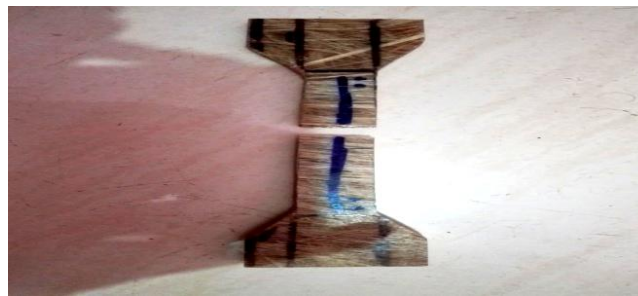
Fig. No 5.2 : Work piece after tensile test
